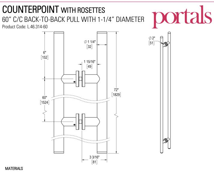
Solid & tubular brass components, stainless steel fasteners, and clear polycarbonate washers
